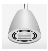
Suspended luminaire with LED, rated life of the LED L80/B10 > 50000 h, colour rendering index CRI > 90, chromaticity tolerance 2 SDCM (initial), reflector with double asymmetrical light distribution pattern, reflector pure aluminium 99,99% in MIRO-Silver®, luminaire housing sheet steel, powder-coated, stratowhite
