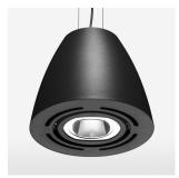
Suspended luminaire with LED, rated life of the LED L80/B10 > 50000 h, colour rendering index CRI > 80, chromaticity tolerance 2 SDCM (initial), reflector with circular light distribution pattern, reflector pure aluminium 99,99% in MIRO-Silver®, swivel angle  $2x25^{\circ}$ , luminaire housing sheet steel, powder-coated, stratoblack
