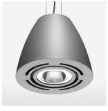
Suspended luminaire with LED, rated life of the LED L80/B10 > 50000 h, colour rendering index CRI > 90, chromaticity tolerance 2 SDCM (initial), reflector with circular light distribution pattern, reflector pure aluminium 99,99% in MIRO-Silver®, swivel angle 2x25°, luminaire housing sheet steel, powder-coated, stratosilver
