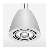
Suspended luminaire with LED, rated life of the LED L80/B10 > 50000 h, chromaticity tolerance 2 SDCM (initial), reflector with circular light distribution pattern, reflector pure aluminium 99,99% in MIRO-Silver®, swivel angle  $2x25^\circ$ , luminaire housing sheet steel, powder-coated, stratowhite
