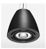
Suspended luminaire with LED, rated life of the LED L80/B10 > 50000 h, colour rendering index CRI > 80, chromaticity tolerance 2 SDCM (initial), reflector with oval light distribution pattern, reflector pure aluminium 99,99% in MIRO-Silver®, swivel angle 2x25°, luminaire housing sheet steel, powder-coated, stratoblack
