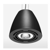
Suspended luminaire with LED, rated life of the LED L80/B10 > 50000 h, colour rendering index CRI > 80, chromaticity tolerance 2 SDCM (initial), reflector with oval light distribution pattern, reflector pure aluminium 99,99% in MIRO-Silver®, swivel angle  $2 \times 25^\circ$ , luminaire housing sheet steel, powder-coated, stratoblack
