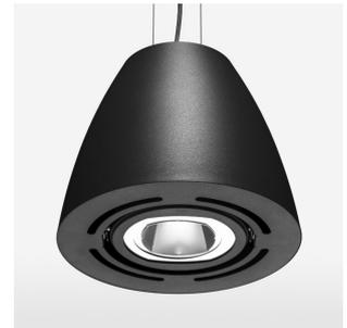
Suspended luminaire with LED, rated life of the LED L80/B10 > 50000 h, colour rendering index CRI > 80, chromaticity tolerance 2 SDCM (initial), reflector with oval light distribution pattern, reflector pure aluminium 99,99% in MIRO-Silver®, swivel angle 2x25°, luminaire housing sheet steel, powder-coated, stratoblack
