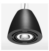
Suspended luminaire with LED, rated life of the LED L80/B10 > 50000 h, colour rendering index CRI > 90, chromaticity tolerance 2 SDCM (initial), reflector with oval light distribution pattern, reflector pure aluminium 99,99% in MIRO-Silver®, swivel angle 2x25°, luminaire housing sheet steel, powder-coated, stratoblack
