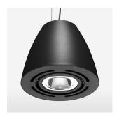
Suspended luminaire with LED, rated life of the LED L80/B10 > 50000 h, chromaticity tolerance 3 SDCM (initial), reflector with oval light distribution pattern, reflector pure aluminium 99,99% in MIRO-Silver®, swivel angle 2x25°, luminaire housing sheet steel, powder-coated, stratoblack
