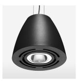
Suspended luminaire with LED, rated life of the LED L80/B10 > 50000 h, chromaticity tolerance 3 SDCM (initial), reflector with oval light distribution pattern, reflector pure aluminium 99,99% in MIRO-Silver®, swivel angle 2x25°, luminaire housing sheet steel, powder-coated, stratoblack
