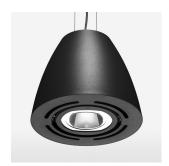
Suspended luminaire with LED, rated life of the LED L80/B10 > 50000 h, chromaticity tolerance 2 SDCM (initial), reflector with circular light distribution pattern, reflector pure aluminium 99,99% in MIRO-Silver®, swivel angle  $2x25^\circ$ , luminaire housing sheet steel, powder-coated, stratoblack
