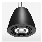
Suspended luminaire with LED, rated life of the LED L80/B10 > 50000 h, colour rendering index CRI > 90, chromaticity tolerance 2 SDCM (initial), reflector with circular light distribution pattern, reflector pure aluminium 99,99% in MIRO-Silver®, swivel angle 2x25°, luminaire housing sheet steel, powder-coated, stratoblack
