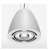
Suspended luminaire with LED, rated life of the LED L80/B10 > 50000 h, chromaticity tolerance 2 SDCM (initial), reflector with circular light distribution pattern, reflector pure aluminium 99,99% in MIRO-Silver®, swivel angle 2x25°, luminaire housing sheet steel, powder-coated, stratowhite
