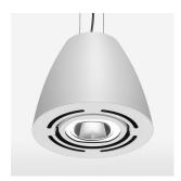
Suspended luminaire with LED, rated life of the LED L80/B10 > 50000 h, chromaticity tolerance 3 SDCM (initial), reflector with circular light distribution pattern, reflector pure aluminium 99,99% in MIRO-Silver®, swivel angle  $2x25^\circ$ , luminaire housing sheet steel, powder-coated, stratowhite
