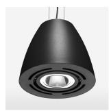
Suspended luminaire with LED, rated life of the LED L80/B10 > 50000 h, colour rendering index CRI > 80, chromaticity tolerance 2 SDCM (initial), reflector with circular light distribution pattern, reflector pure aluminium 99,99% in MIRO-Silver®, swivel angle 2x25°, luminaire housing sheet steel, powder-coated, stratoblack
