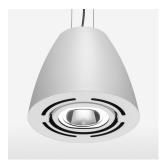
Suspended luminaire with LED, rated life of the LED L80/B10 > 50000 h, chromaticity tolerance 2 SDCM (initial), reflector with circular light distribution pattern, reflector pure aluminium 99,99% in MIRO-Silver®, swivel angle  $2 \times 25^\circ$ , luminaire housing sheet steel, powder-coated, stratowhite
