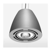
Suspended luminaire with LED, rated life of the LED L80/B10 > 50000 h, colour rendering index CRI > 80, chromaticity tolerance 2 SDCM (initial), reflector with oval light distribution pattern, reflector pure aluminium 99,99% in MIRO-Silver®, swivel angle  $2 \times 25^\circ$ , luminaire housing sheet steel, powder-coated, stratosilver
