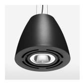
Suspended luminaire with LED, rated life of the LED L80/B10 > 50000 h, chromaticity tolerance 2 SDCM (initial), reflector with oval light distribution pattern, reflector pure aluminium 99,99% in MIRO-Silver®, swivel angle  $2x25^{\circ}$ , luminaire housing sheet steel, powder-coated, stratoblack
