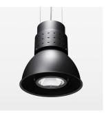
Suspended luminaire with LED, rated life of the LED L80/B10 > 50000 h, colour rendering index CRI > 80, chromaticity tolerance 2 SDCM (initial), reflector with circular light distribution pattern, reflector pure aluminium 99,99% in MIRO-Silver®, luminaire shade die-cast aluminium, powdercoated, swivel angle +25°/-25°, luminaire housing sheet steel, powder-coated, stratoblack
