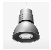
Suspended luminaire with LED, rated life of the LED L80/B10 > 50000 h, chromaticity tolerance 3 SDCM (initial), reflector with circular light distribution pattern, reflector pure aluminium 99,99% in MIRO-Silver®, luminaire shade die-cast aluminium, powder-coated, swivel angle +25°/-25°, luminaire housing sheet steel, powder-coated, stratosilver
