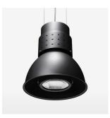
Suspended luminaire with LED, rated life of the LED L80/B10 > 50000 h, chromaticity tolerance 3 SDCM (initial), reflector with oval light distribution pattern, reflector pure aluminium 99,99% in MIRO-Silver®, luminaire shade die-cast aluminium, powder-coated, swivel angle +25°/-25°, luminaire housing sheet steel, powder-coated, stratoblack
