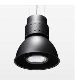
Suspended luminaire with LED, rated life of the LED L80/B10 > 50000 h, chromaticity tolerance 3 SDCM (initial), reflector with circular light distribution pattern, reflector pure aluminium 99,99% in MIRO-Silver®, luminaire shade die-cast aluminium, powder-coated, swivel angle +25°/-25°, luminaire housing sheet steel, powder-coated, stratoblack
