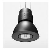
Suspended luminaire with LED, rated life of the LED L80/B10 > 50000 h, colour rendering index CRI > 90, chromaticity tolerance 2 SDCM (initial), reflector with double asymmetrical light distribution pattern, reflector pure aluminium 99,99% in MIRO-Silver®, luminaire shade die-cast aluminium, powder-coated, luminaire housing sheet steel, powder-coated, stratoblack
