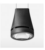
Suspended luminaire with LED, rated life of the LED L80/B10 > 50000 h, colour rendering index CRI > 80, chromaticity tolerance 2 SDCM (initial), reflector with circular light distribution pattern, reflector pure aluminium 99,99% in MIRO-Silver®, luminaire head die-cast aluminium, powder-coated, stratoblack
