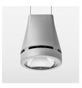
Suspended luminaire with LED, rated life of the LED L80/B10 > 50000 h, colour rendering index CRI > 90, chromaticity tolerance 2 SDCM (initial), reflector with circular light distribution pattern, reflector pure aluminium 99,99% in MIRO-Silver®, luminaire head die-cast aluminium, powder-coated, stratosilver
