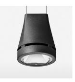
Suspended luminaire with LED, rated life of the LED L80/B10 > 50000 h, colour rendering index CRI > 90, chromaticity tolerance 2 SDCM (initial), reflector with circular light distribution pattern, reflector pure aluminium 99,99% in MIRO-Silver®, luminaire head die-cast aluminium, powder-coated, stratoblack
