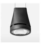
Suspended luminaire with LED, rated life of the LED L80/B10 > 50000 h, chromaticity tolerance 3 SDCM (initial), reflector with circular light distribution pattern, reflector pure aluminium 99,99% in MIRO-Silver®, luminaire head die-cast aluminium, powder-coated, stratoblack
