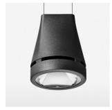
Suspended luminaire with LED, rated life of the LED L80/B10 > 50000 h, colour rendering index CRI > 80, chromaticity tolerance 2 SDCM (initial), reflector with circular light distribution pattern, reflector pure aluminium 99,99% in MIRO-Silver®, luminaire head die-cast aluminium, powder-coated, stratoblack
