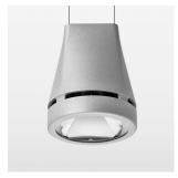
Suspended luminaire with LED, rated life of the LED L80/B10 > 50000 h, colour rendering index CRI > 90, chromaticity tolerance 2 SDCM (initial), reflector with circular light distribution pattern, reflector pure aluminium 99,99% in MIRO-Silver®, luminaire head die-cast aluminium, powder-coated, stratosilver
