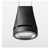
Suspended luminaire with LED, rated life of the LED L80/B10 > 50000 h, colour rendering index CRI > 80, chromaticity tolerance 2 SDCM (initial), reflector with oval light distribution pattern, reflector pure aluminium 99,99% in MIRO-Silver®, luminaire head die-cast aluminium, powder-coated, stratoblack
