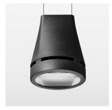
Suspended luminaire with LED, rated life of the LED L80/B10 > 50000 h, colour rendering index CRI > 90, chromaticity tolerance 2 SDCM (initial), reflector with oval light distribution pattern, reflector pure aluminium 99,99% in MIRO-Silver®, luminaire head die-cast aluminium, powder-coated, stratoblack
