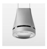
Suspended luminaire with LED, rated life of the LED L80/B10 > 50000 h, colour rendering index CRI > 90, chromaticity tolerance 2 SDCM (initial), reflector with oval light distribution pattern, reflector pure aluminium 99,99% in MIRO-Silver®, luminaire head die-cast aluminium, powder-coated, stratosilver
