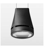
Suspended luminaire with LED, rated life of the LED L80/B10 > 50000 h, chromaticity tolerance 2 SDCM (initial), reflector with oval light distribution pattern, reflector pure aluminium 99,99% in MIRO-Silver®, luminaire head die-cast aluminium, powder-coated, stratoblack
