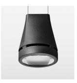
Suspended luminaire with LED, rated life of the LED L80/B10 > 50000 h, chromaticity tolerance 3 SDCM (initial), reflector with oval light distribution pattern, reflector pure aluminium 99,99% in MIRO-Silver®, luminaire head die-cast aluminium, powder-coated, stratoblack
