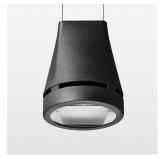
Suspended luminaire with LED, rated life of the LED L80/B10 > 50000 h, chromaticity tolerance 2 SDCM (initial), reflector with oval light distribution pattern, reflector pure aluminium 99,99% in MIRO-Silver®, luminaire head die-cast aluminium, powder-coated, stratoblack
