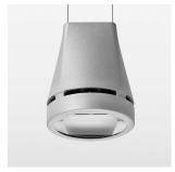
Suspended luminaire with LED, rated life of the LED L80/B10 > 50000 h, chromaticity tolerance 2 SDCM (initial), reflector with oval light distribution pattern, reflector pure aluminium 99,99% in MIRO-Silver®, luminaire head die-cast aluminium, powder-coated, stratosilver
