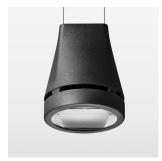
Suspended luminaire with LED, rated life of the LED L80/B10 > 50000 h, chromaticity tolerance 3 SDCM (initial), reflector with oval light distribution pattern, reflector pure aluminium 99,99% in MIRO-Silver®, luminaire head die-cast aluminium, powder-coated, stratoblack
