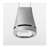
Suspended luminaire with LED, rated life of the LED L80/B10 > 50000 h, colour rendering index CRI > 80, chromaticity tolerance 2 SDCM (initial), reflector with circular light distribution pattern, reflector pure aluminium 99,99% in MIRO-Silver®, luminaire head die-cast aluminium, powder-coated, stratosilver
