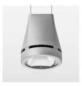
Suspended luminaire with LED, rated life of the LED L80/B10 > 50000 h, colour rendering index CRI > 80, chromaticity tolerance 2 SDCM (initial), reflector with circular light distribution pattern, reflector pure aluminium 99,99% in MIRO-Silver®, luminaire head die-cast aluminium, powder-coated, stratosilver
