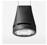
Suspended luminaire with LED, rated life of the LED L80/B10 > 50000 h, chromaticity tolerance 3 SDCM (initial), reflector with circular light distribution pattern, reflector pure aluminium 99,99% in MIRO-Silver®, luminaire head die-cast aluminium, powder-coated, stratoblack
