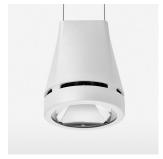
Suspended luminaire with LED, rated life of the LED L80/B10 > 50000 h, chromaticity tolerance 2 SDCM (initial), reflector with circular light distribution pattern, reflector pure aluminium 99,99% in MIRO-Silver®, canopy sheet steel, powder-coated, luminaire head die-cast aluminium, powder-coated, stratowhite
