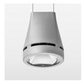
Suspended luminaire with LED, rated life of the LED L80/B10 > 50000 h, chromaticity tolerance 2 SDCM (initial), reflector with circular light distribution pattern, reflector pure aluminium 99,99% in MIRO-Silver®, canopy sheet steel, powder-coated, luminaire head die-cast aluminium, powder-coated, stratosilver
