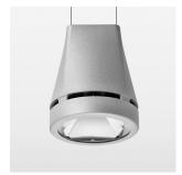
Suspended luminaire with LED, rated life of the LED L80/B10 > 50000 h, colour rendering index CRI > 90, chromaticity tolerance 2 SDCM (initial), reflector with circular light distribution pattern, reflector pure aluminium 99,99% in MIRO-Silver®, canopy sheet steel, powder-coated, luminaire head die-cast aluminium, powder-coated, stratosilver
