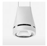
Suspended luminaire with LED, rated life of the LED L80/B10 > 50000 h, chromaticity tolerance 2 SDCM (initial), reflector with circular light distribution pattern, reflector pure aluminium 99,99% in MIRO-Silver®, canopy sheet steel, powder-coated, luminaire head die-cast aluminium, powder-coated, stratowhite
