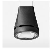
Suspended luminaire with LED, rated life of the LED L80/B10 > 50000 h, chromaticity tolerance 3 SDCM (initial), reflector with circular light distribution pattern, reflector pure aluminium 99,99% in MIRO-Silver®, canopy sheet steel, powder-coated, luminaire head die-cast aluminium, powder-coated, stratoblack
