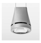
Suspended luminaire with LED, rated life of the LED L80/B10 > 50000 h, chromaticity tolerance 2 SDCM (initial), reflector with circular light distribution pattern, reflector pure aluminium 99,99% in MIRO-Silver®, canopy sheet steel, powder-coated, luminaire head die-cast aluminium, powder-coated, stratosilver
