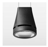
Suspended luminaire with LED, rated life of the LED L80/B10 > 50000 h, chromaticity tolerance 2 SDCM (initial), reflector with oval light distribution pattern, reflector pure aluminium 99,99% in MIRO-Silver®, canopy sheet steel, powder-coated, luminaire head die-cast aluminium, powder-coated, stratoblack
