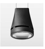
Suspended luminaire with LED, rated life of the LED L80/B10 > 50000 h, colour rendering index CRI > 90, chromaticity tolerance 2 SDCM (initial), reflector with oval light distribution pattern, reflector pure aluminium 99,99% in MIRO-Silver®, canopy sheet steel, powder-coated, luminaire head die-cast aluminium, powder-coated, stratoblack
