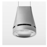
Suspended luminaire with LED, rated life of the LED L80/B10 > 50000 h, chromaticity tolerance 2 SDCM (initial), reflector with oval light distribution pattern, reflector pure aluminium 99,99% in MIRO-Silver®, canopy sheet steel, powder-coated, luminaire head die-cast aluminium, powder-coated, stratosilver
