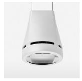
Suspended luminaire with LED, rated life of the LED L80/B10 > 50000 h, chromaticity tolerance 3 SDCM (initial), reflector with oval light distribution pattern, reflector pure aluminium 99,99% in MIRO-Silver®, canopy sheet steel, powder-coated, luminaire head die-cast aluminium, powder-coated, stratowhite
